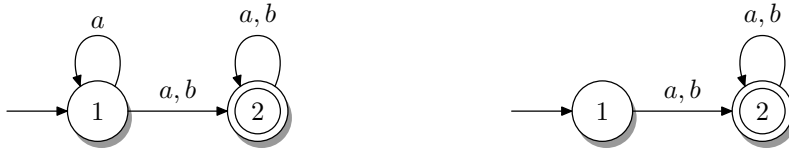
Fig. 1. The NFA A (left) and the minimal DFA (right) accepting the language L(A) . The transition monoid of A has size 3, while the transition monoid, which is equivalent to the syntactic monoid of L(A) , contains only 2 elements.
